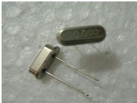
Figure 3.3: Quartz de 20 MHz
